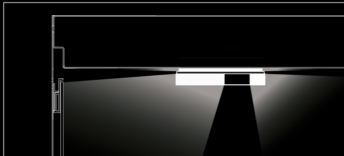
Vertical section of LD7-NEO-LED wallwasher. Functional diagram of direct and indirect lighting.
