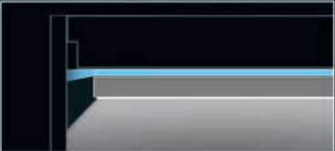
Vertical section: LD8-LED-RGB ceiling light. Functional diagram of direct lighting. LED neutral white, LED-RGB lighting control.
