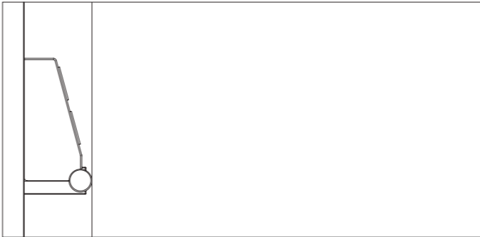
Vertical section: side wall, control panel EN 81-70-B.
