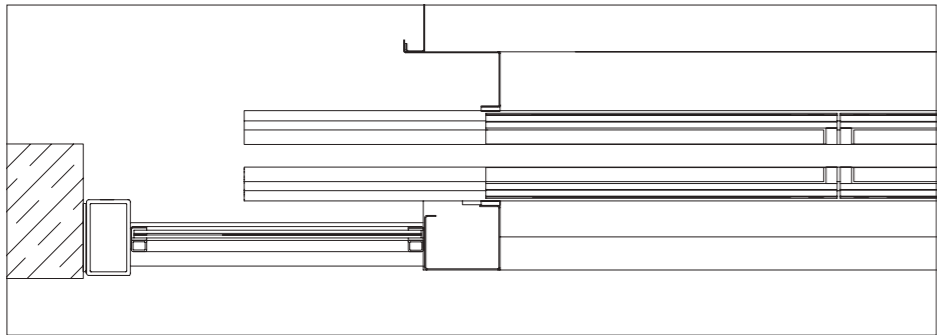
Horizontal section: car and landing door, All-glass door with glass portal P7-G
