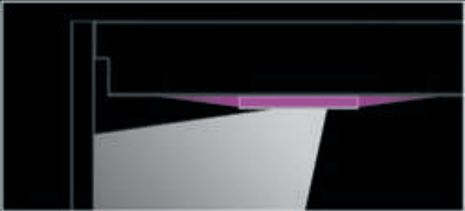
Vertical section of LD7 LED RGB wallwasher Functional diagram of direct and indirect lighting
