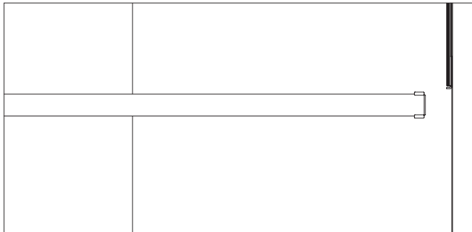
Vertical section of rear wall / mirror S5, surface-mounted.
