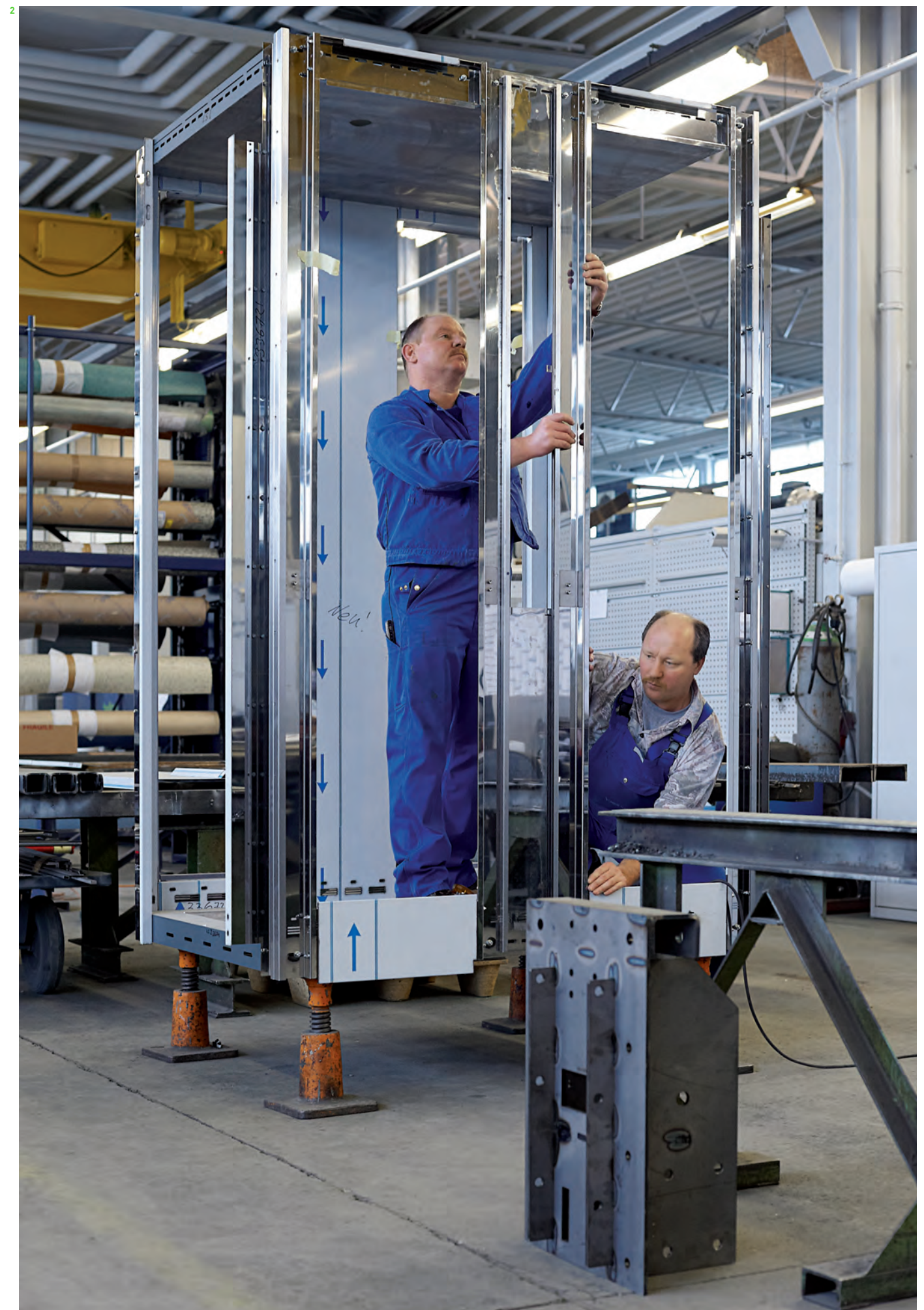
2 Car installation for a glass panorama lift
